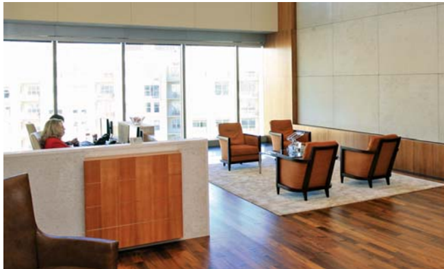
Lobby — Koa wood, Hawaiian lumber that has not been harvested but collected from forest floors after falling, is used throughout the office, including as a component of the two-story reception area walls.
