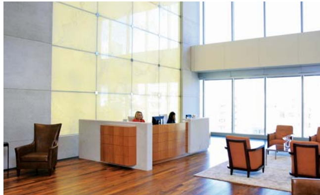
Lobby — The onyx feature wall is backlit by low-voltage LED light sources. The firm selected reclaimed teak for elevator lobbies and the main reception area.
